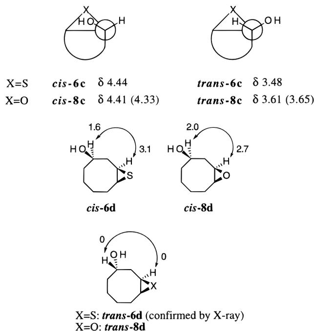
**Figure 1.** Characteristic  $\delta_{\text{H}}(\text{CH}-\text{OH})$  data and NOE effects (%) of selected thiranes **6** and epoxides **8**, in parentheses data from ref 21.
